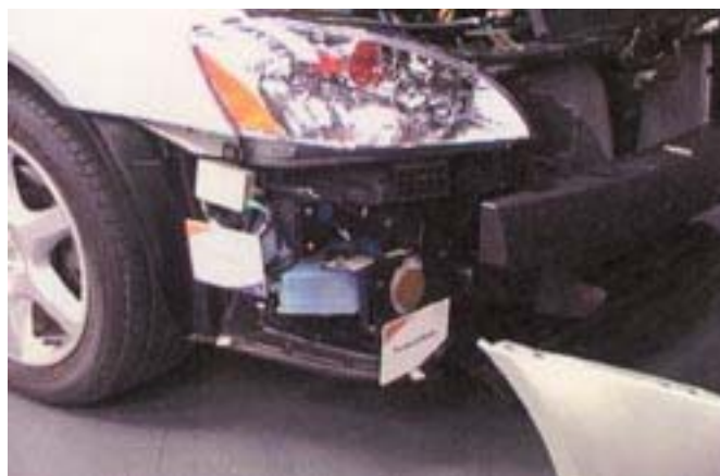
Forward and side facing radar units are mounted at the front corners of the vehicle behind the fascia.
